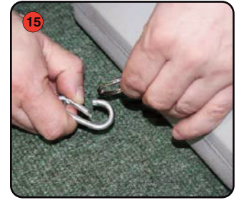
Attach the base springs to each base tank ring.
